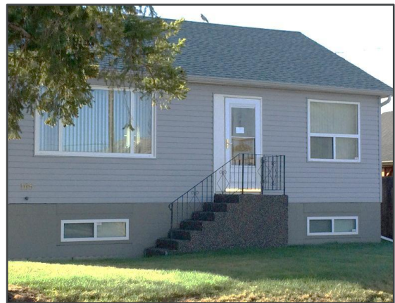
For this house, the setback from the property line is measured from the house, while the steps leading to the front door project or intrude into the setback area
